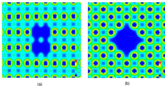
FIG. 2: (a) Contours of electron-density around a planar quad-vacancy (Configuration No. 5 in Table 1) on  $\{110\}$  plane in a million atom sample. This planar quad-vacancy has the highest binding energy among the various quad-vacancies considered. (b) Contours of electron-density around a planar quad-vacancy (Configuration No. 1 in Table 1) on  $\{100\}$  plane in a million atom sample.
