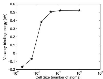
FIG. 3: Cell-size dependence of vacancy binding energy for the quad-vacancy given by the first configuration in Table I.
